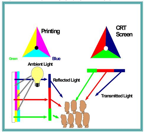
Figure 3 Differences between Reflected and Transmitted Light
