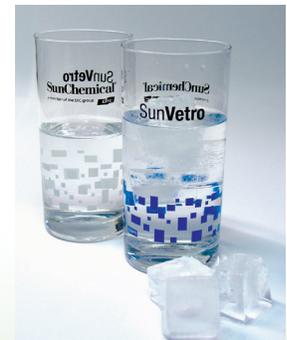
**Figure 2** Thermochromic inks were applied to these glasses. Colder temperatures change the color of the ink from white to blue.
