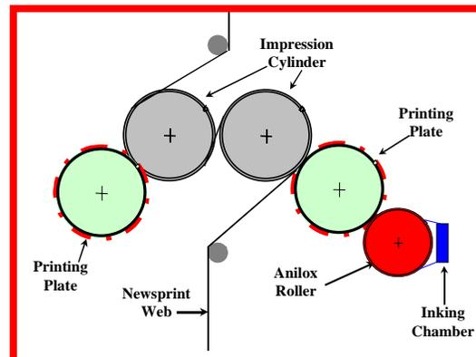
engraving pattern, which allows a specific volume of ink to be transferred to the printing plate. The anilox cylinder has a scraper (doctor) blade that removes any excess ink from the anilox cylinder and returns it to the ink fountain. The image is then transferred directly from the printing plate onto the surface of the newsprint. This process requires a “kiss” impression for uniform printing.
