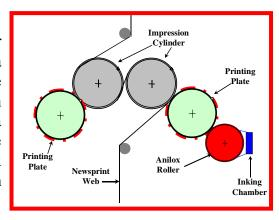
engraving pattern, which allows a specific volume of ink to be transferred to the printing plate. The anilox cylinder has a scraper (doctor) blade that removes any excess ink from the anilox cylinder and returns it to the ink fountain. The image is then transferred directly from the printing plate onto the surface of the newsprint. This process requires a "kiss" impression for uniform printing.
