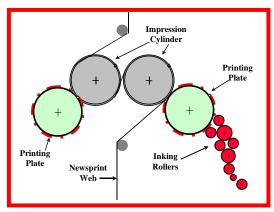
and uniformly. The impression cylinder is covered with a hard rubber material that can withstand numerous impressions. The printing of the two sides of the web is done at different times.
