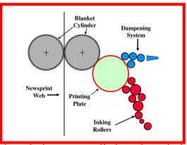
an oil based ink and a water based fountain solution are applied to the printing plate. The fountain solution wets the non-image area of the plate while the ink wets the image area.
