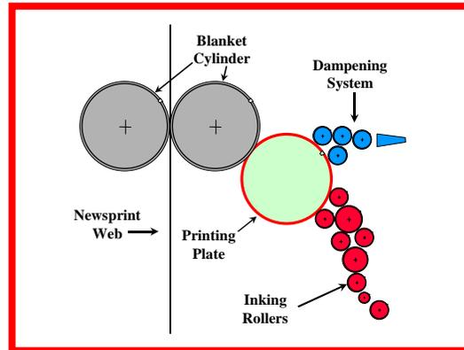
The ink is applied to the printing plate through a series of rollers. These rollers serve to thin the ink film so the proper amount is applied to the plate. The fountain solution can be applied in several different ways: the solution can be sprayed on, transferred from a high-speed brush or by a molleton or sock roller.
