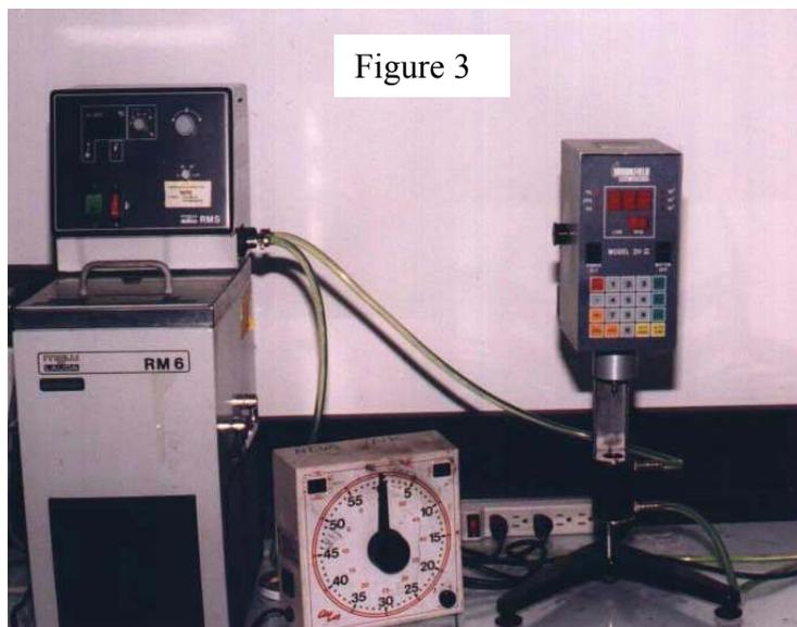
Viscosity is a very complex property of ink and it is critical that similar **methods and equipment** are utilized in comparing ink viscosity. Viscosity is the scientific term for resistance to flow. For a more in-depth look at the study of viscosity, see the technical bulletin Volume VII. The most common instrument used in the news ink industry to measure viscosity, is a Brookfield viscometer with a small
