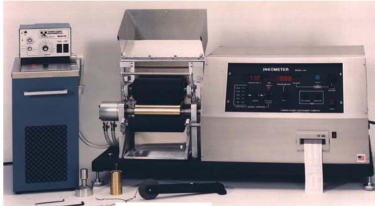
separating surfaces. Tack is a critical property used to control the ink's tendency to pull lint from the newsprint. Figure 4
