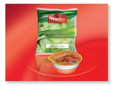
The SunLase solution prints a transparent or tinted coating onto a packaging substrate during the printing process. After the packaging has been sealed, variable coding graphic information, such as barcodes, QR codes, and "Use By" dates, can be created using a low power  $CO_2$  or fibre laser to change the colour of the patch to black where marked, with no risks to the packaged product.
