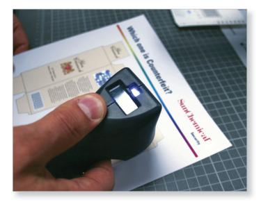
The SunLock<sup>®</sup> Verigard<sup>™</sup> solution is one of the most sophisticated anti-counterfeiting measures available on the market. It tunes a proprietary reader to look for a unique taggant signature or multiple signatures, making it extremely secure on packaging.
