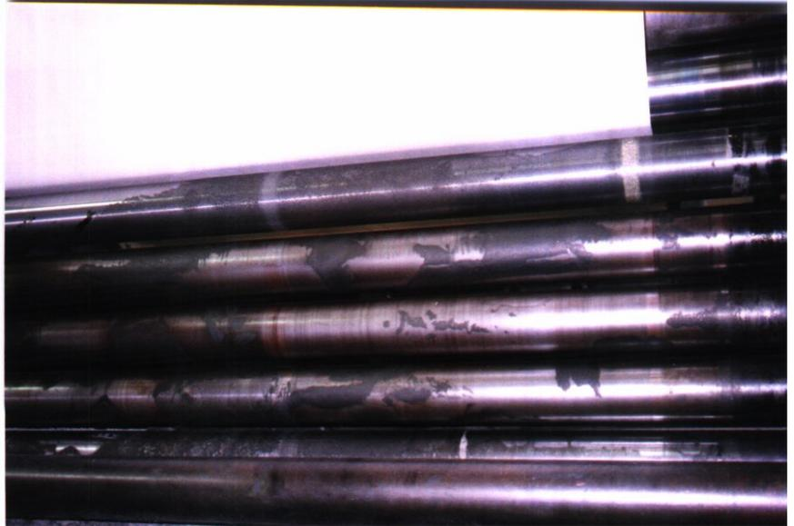
Build up may be soft and readily removable, or hard and difficult to remove. There are several causes of build up, let's try to identify which are relevant to the problem
