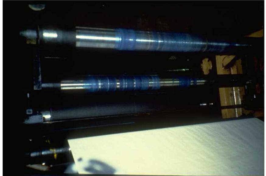
If that is unacceptable, and time permits then extra cleaning of the relevant rollers/bars may be considered the only solution. If it can be predicted from past experience that a
