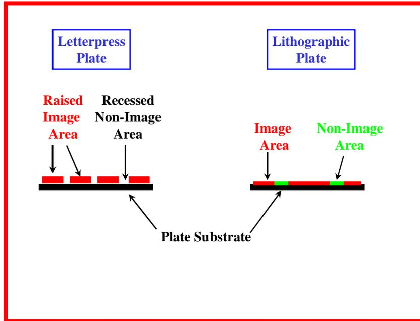
This section is a generalization of the types of printing processes for newspapers. Various manufacturers of printing presses utilize different designs for their presses. The intention of this section is to give an overview of the processes so that one can contrast the differences.
