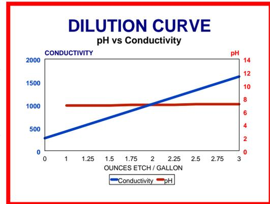
The level of conductivity of a solution is measured with a conductivity meter, which gives readings in micromhos. As a rule, conductivity meters are accurate, easy to calibrate, and simple to use. They are operated simply by either dipping the electrode into the solution and stirring for a few seconds to obtain a reading, or pouring the fountain solution into a cup and then getting the reading.
