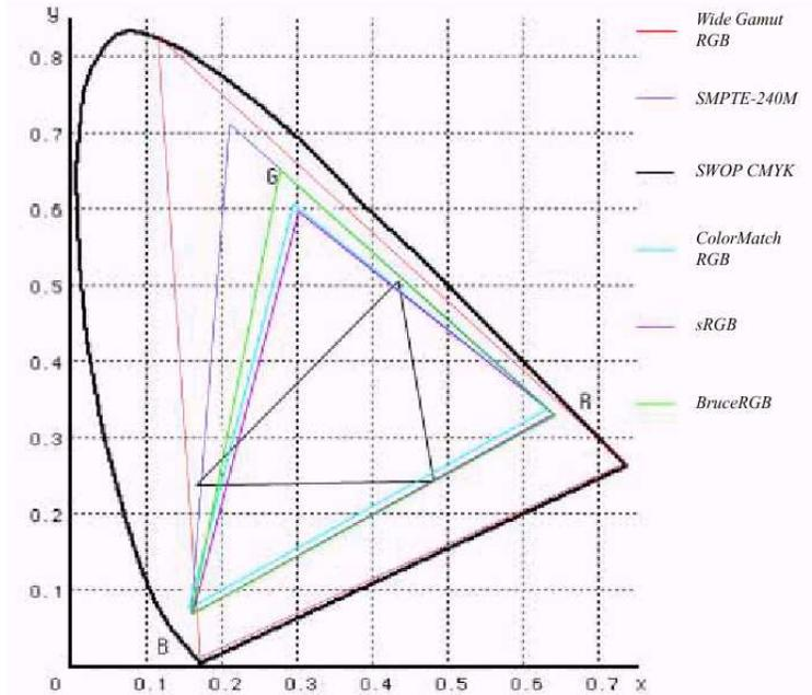
*This figure shows the gamuts of several of Photoshop's working RGB spaces, and the gamut of SWOP CMYK, plotted in CIE xyY space. It illustrates the trade-off inherent in choosing an RGB space between clipping the gamut of CMYK and wasting bits on unprintable colors.*
