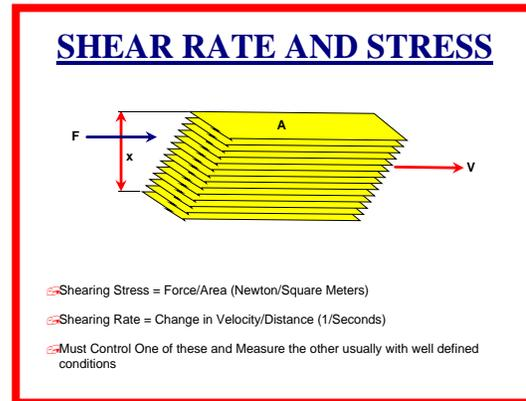
Even though a fluid can deform easily under an applied force, the fluid's viscosity creates resistance to this force. Viscosity can be appreciated by visualizing a cube of fluid between two plates as shown in the above figure. If a shearing force (F) is
