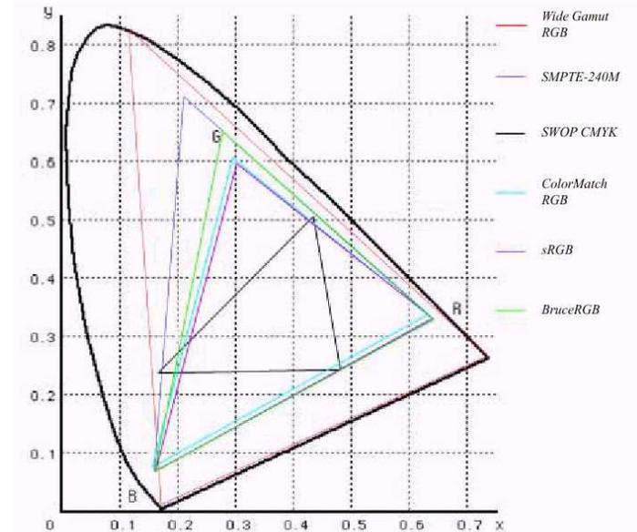
*This figure shows the gamuts of several of Photoshop's working RGB spaces, and the gamut of SWOP CMYK, plotted in CIE xyY space. It illustrates the trade-off inherent in choosing an RGB space between clipping the gamut of CMYK and wasting bits on unprintable colors.*
