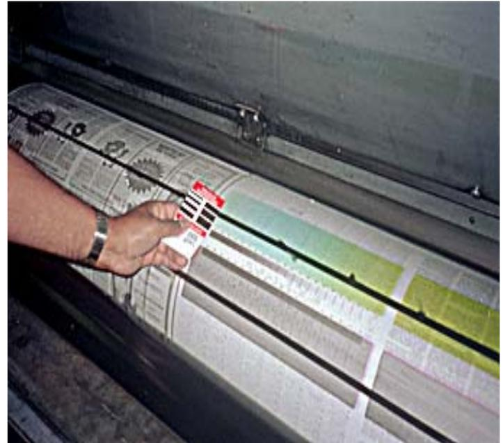
Proper setting begins with the [ductor](#)
