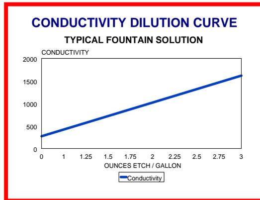
Conductivity is the ability to transmit or conduct an electrical charge. In solutions, the conductivity is determined by the number of ions present in solution (see figure 3.) Basically, the higher the level of fountain solution concentrate used in the solution, the higher the conductivity will be. Figure 4 shows a typical conductivity vs. pH curve for a fountain solution. As you can see from the graph,
