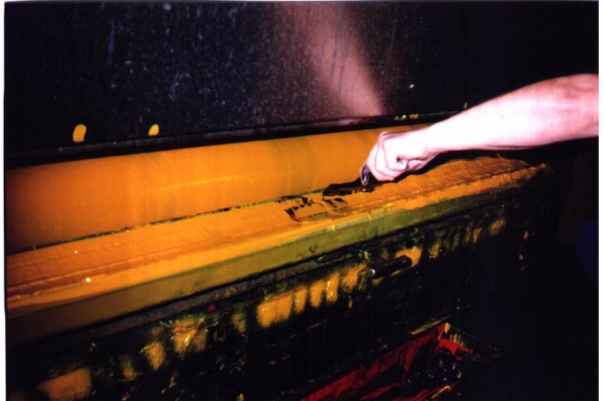
to the method of storage and handling. A difficulty often arises where ink has necessarily been formulated with short flow for manual handling, but this leads to a tendency towards hanging back. In such a case an automatic fountain agitator is a
