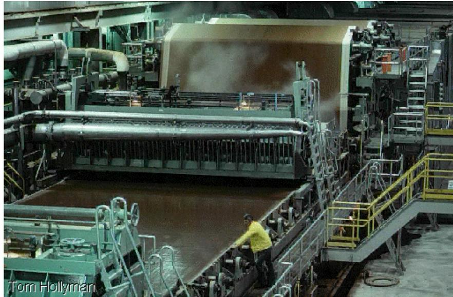
(typically 1% fibers and 99% water) uniformly onto a continuously running wire. The fibers orientate themselves on the wire and the water drains through and is
