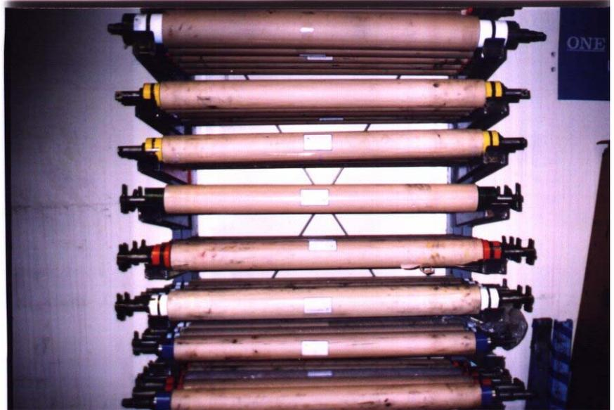
cleaning and refinishing process, roller should be stored vertically in racks enclosed in a cabinet. Horizontal racks are satisfactory for short rollers, but vertical storage is recommended. Long rollers should be stored vertically, to avoid
