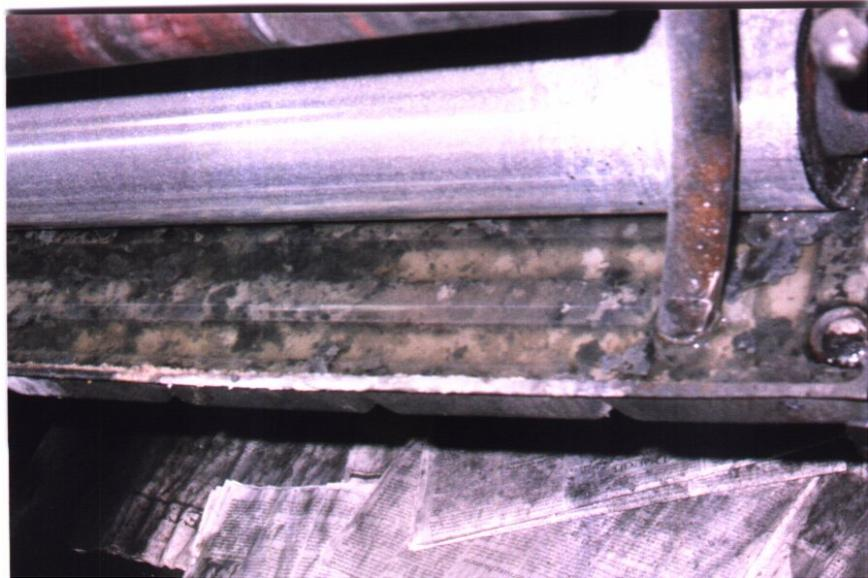
3. When removing plates and before putting on new plates, the plate cylinder should be checked and cleaned.
