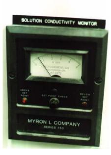
solution. To ensure that you comply with the fountain solution manufacturers recommendations make a note of the conductivity which corresponds to the desired dilution and use this figure for control purposes. If the incoming water supply or fountain solution concentrate change then this standard dilution test must be repeated. It is important to test the pH also since all fountain solutions are not buffered.
