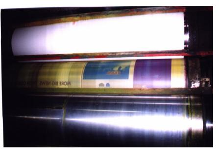
then the remaining ink is to be removed with a suitable <u>wash</u>. There are many suitable washes available but unfortunately also many unsuitable ones. To be avoided are all polar solvents such as esters, keytones, and chlorinated washes. These are not only harmful to the blanket as they swell the face rubber and remove chemicals necessary to
