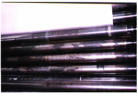
Build up may be soft and readily removable, or hard and difficult to remove. There are several causes of build up, lets try to identify which are relevant to the problem
