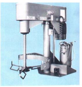
The most commonly used equipment for premixing and pre-dispersion work is a high-speed disperser. These types of dispersers are most commonly found in ink manufacturing sites. They may have a variable, dual, or fixed speed drive.
