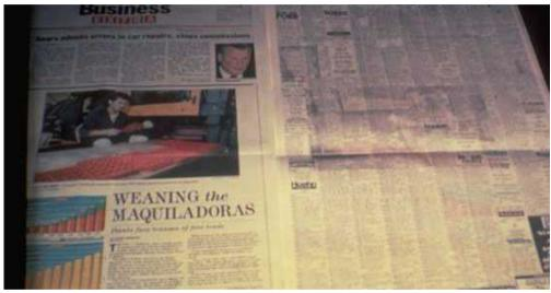
causes of marking, lets try to identify which is relevant to the problem observed. Marking is a cumulative problem, and thus relates to length of run and period between cleaning of the relevant press equipment. Have the affected units been cleaned according to their normal pattern? Obviously that should be easy to
