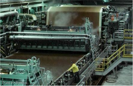
(typically 1% fibers and 99% water) uniformly onto a continuously running wire. The fibers orientate themselves on the wire and the water drains through and is
