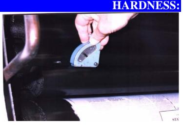
indenter point under spring tension. The harder the material, the higher the reading. The "A" is the most popular Shore instrument, but there are several
