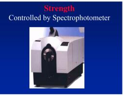
the standard can more easily be seen by the naked eye. The use of color spectrophotometers can be used to quantify the bleach results and to measure shade differences. A color spectrophotometer is an instrument that measures reflectance within the visible spectrum of a sample.
