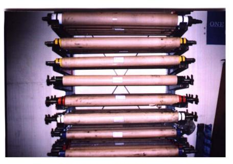
cleaning and refinishing process, roller should be stored vertically in racks enclosed in a cabinet. Horizontal racks are satisfactory for short rollers, but vertical storage is recommended. Long rollers should be stored vertically, to avoid
