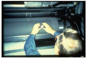
What this means to a printer is that all blankets lose some thickness immediately, called setting in, and then continue to lose thickness throughout the life of the blanket. The initial loss is not only unavoidable but also necessary since during this period the blanket settles in absorbing unevenness in the packing, the press and the blanket itself.
