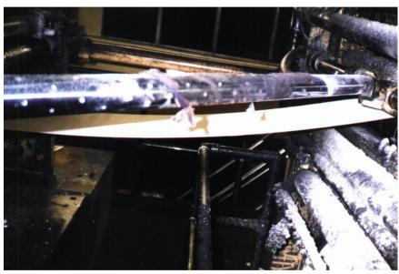
debris on the surface. This is a classic cause of lint, which will appear as a paperlike, thin, very even deposit on the blanket. (this should not be confused with blanket build up, which originates from the ink, and is uneven, often hard and
