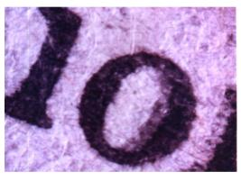
Too much ink being run. - Reduce ink feed. Incorrect plate/blanket packing. Check packing and adjust as required.
