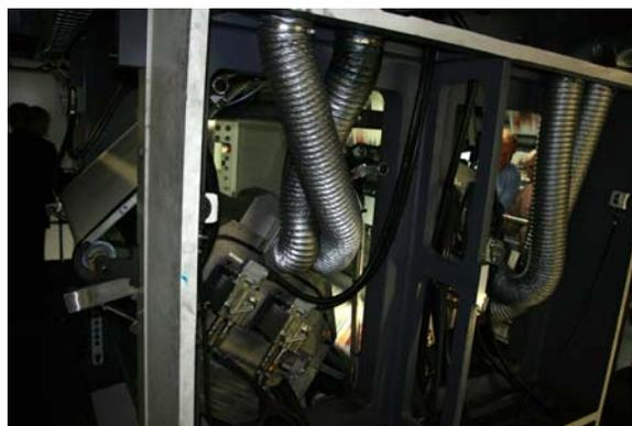
Also the ozone created from the mercury lamps will need to be exhausted into the atmosphere outside of the work area. Emitting ozone into the atmosphere is not a bad thing, but high ozone levels in an enclosed area can cause some health and safety issues – particularly respiratory concerns. This is why the EPA often uses the catch phrase **“good up high, bad nearby.”**
