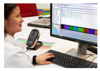
SunColorQC is a software platform hosted on the Sun Chemical network that uses software and a connected spectrophotometer to measure the quality of the output on press.
