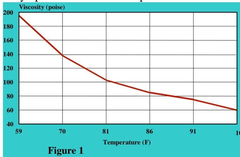
range of most web offset printing presses. However, since viscosity is dependent on temperature, it is important to recognize that a large fluctuation in temperature can change viscosity and ultimately the ink
