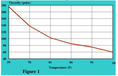
range of most web offset printing presses. However, since viscosity is dependent on temperature, it is important to recognize that a large fluctuation in temperature can change viscosity and ultimately the ink
