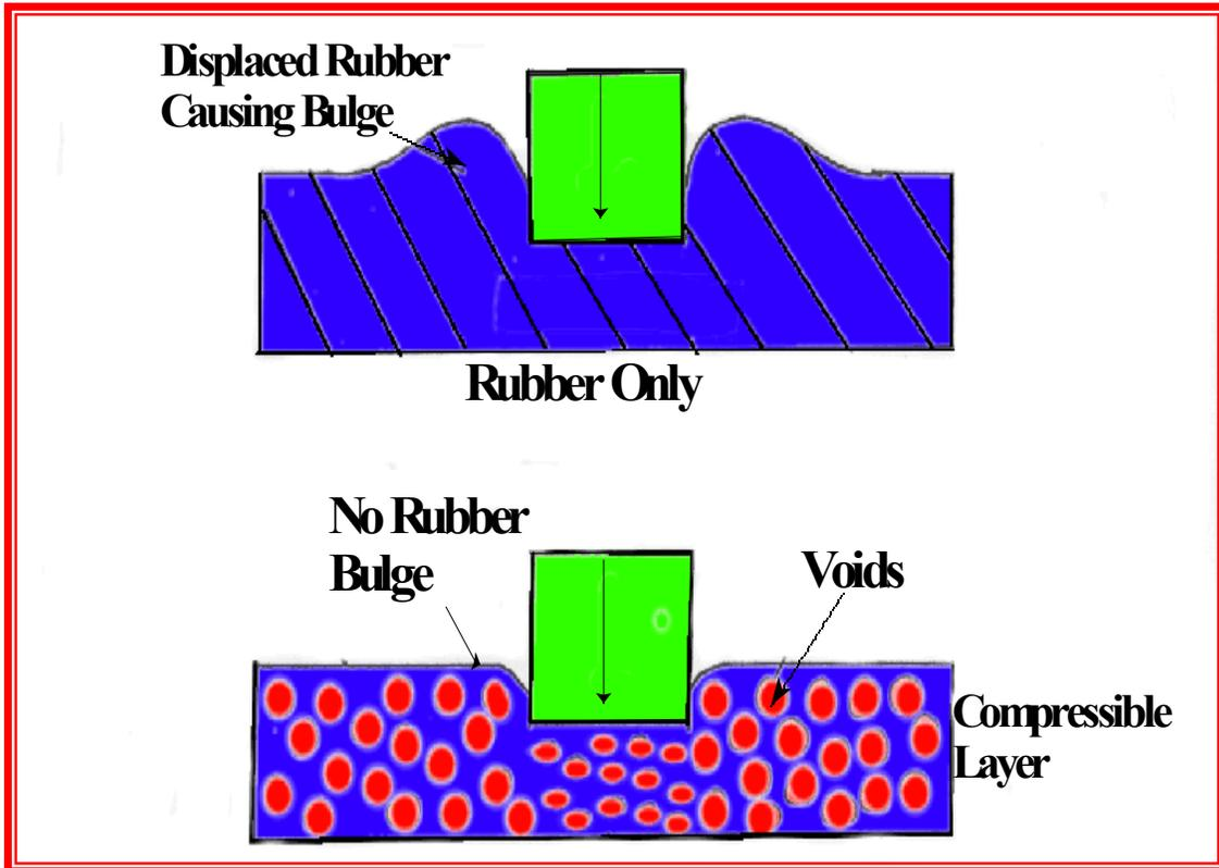
**Figure 1** Compressible Layer Function
