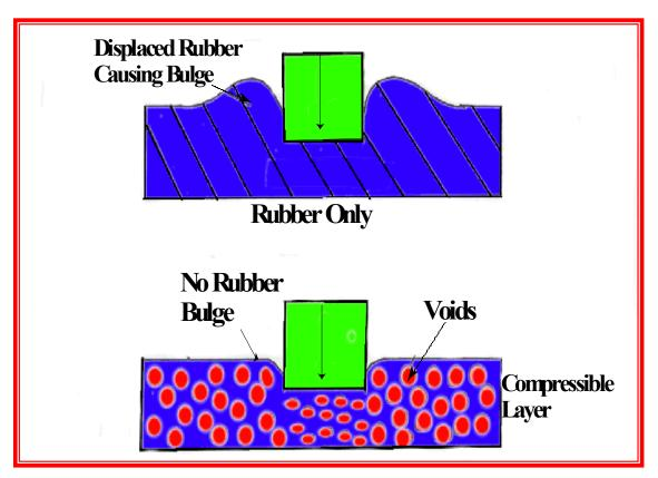
Figure 1Compressible Layer Function
