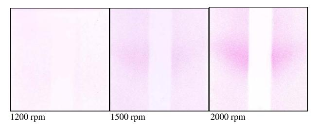
The above images show the impact, under controlled conditions, of the level of misting that occurs during the same time period. One can easily see that as the RPMs increase so does the level of misting. One can look at the above example and may deduce that the higher RPM condition has more splits per unit time and that the lower RPM will create the same level of mist as the time normalizes.
