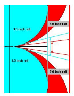
Another important factor to understand is that with smaller rollers the exit nip has a greater angle and shorter depth of the film splitting area. Figure 2 shows the roller splitting differences between a 3.5 inch and a 5.5 inch set of rollers. One can clearly see that the angle exiting the nip of the smaller rollers is greater than the larger rollers.
